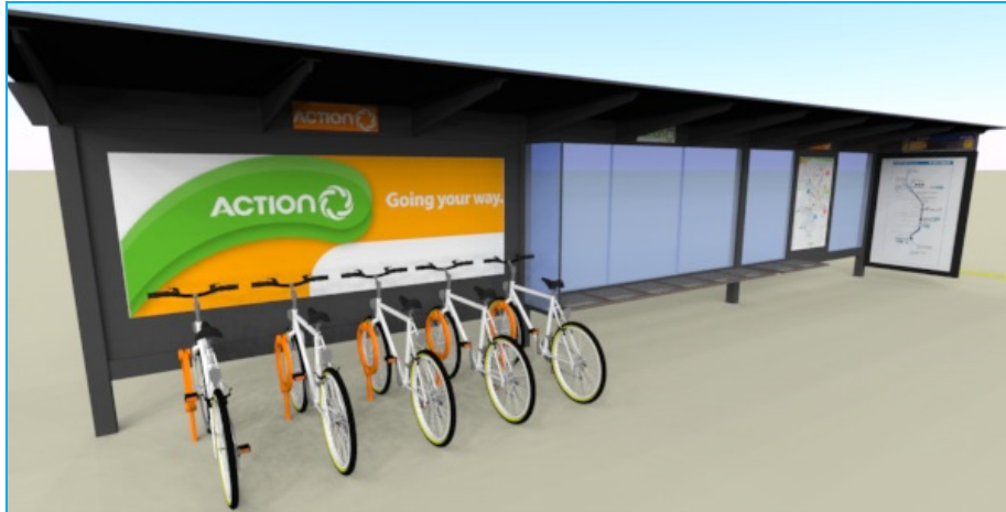
Figure 4.2: Casual Bike Racks Integrated into Bus Shelter (Proposed Modification to Existing Shelter Design)
